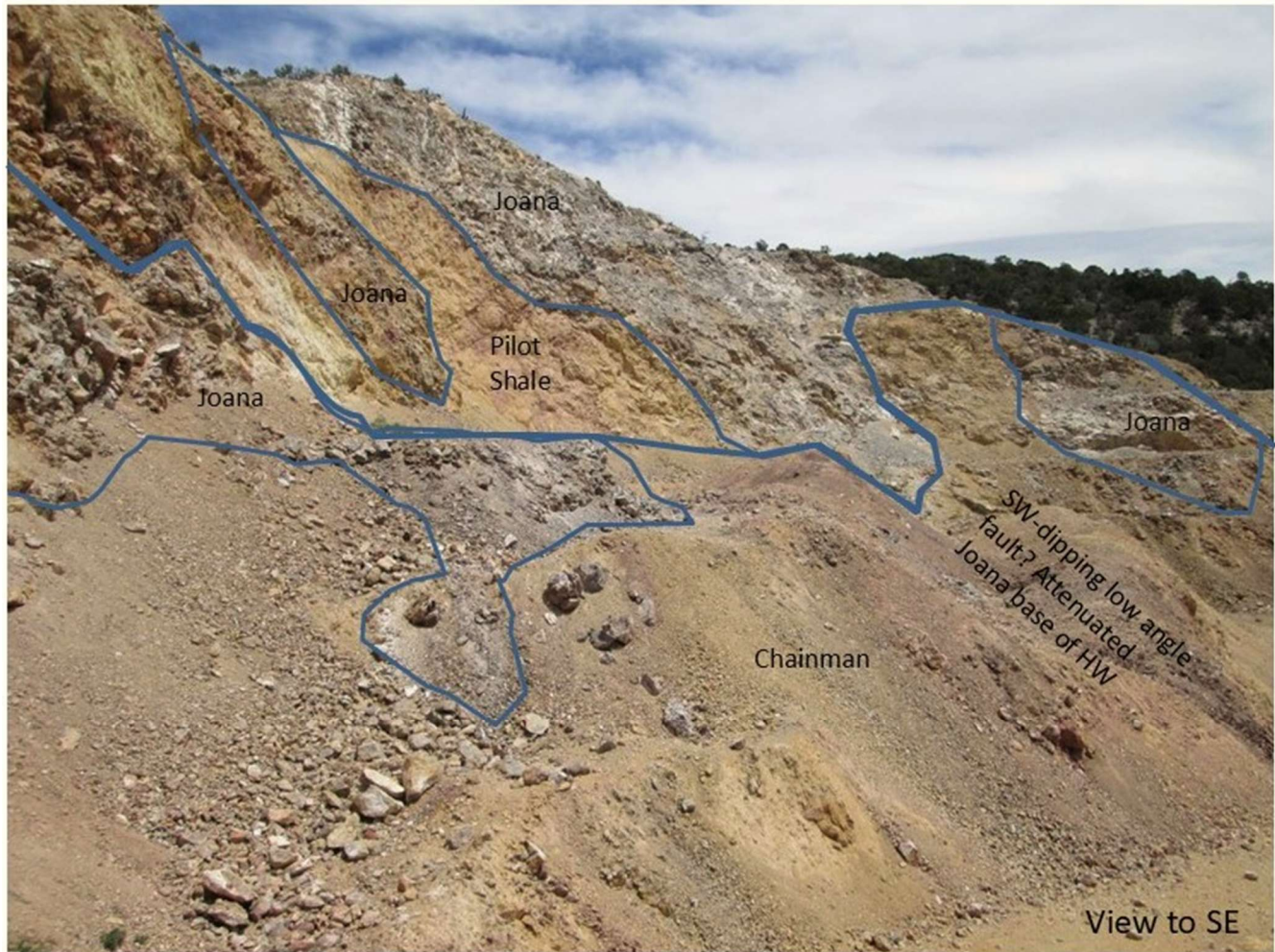
Figure 5: Discovery Ridge Pit showing delineation between the Pilot Shale, Chainman Shale and the Joana Limestone formations (Source: Pilot Gold (USA) Inc., 2013)
