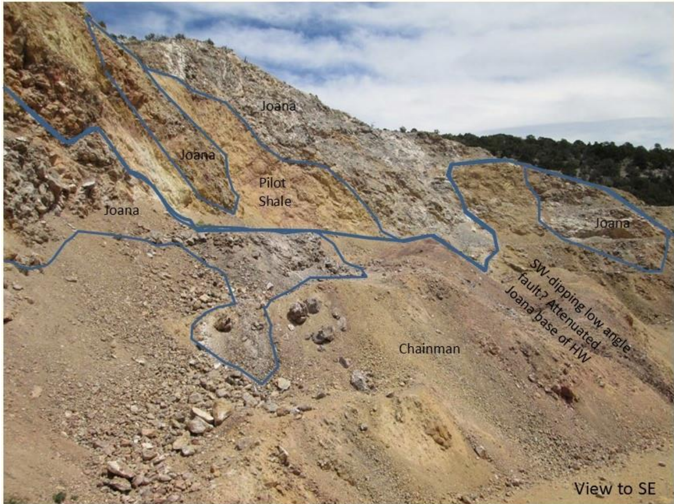
Figure 3: Discovery Ridge Pit showing delineation between the Pilot Shale, Chainman Shale and the Joana Limestone formations (Source: Pilot Gold (USA) Inc., 2013)
