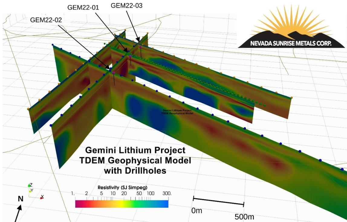
***Geophysical TDEM Model Showing Conductive Zones and 2022 Drill Holes at Gemini***
