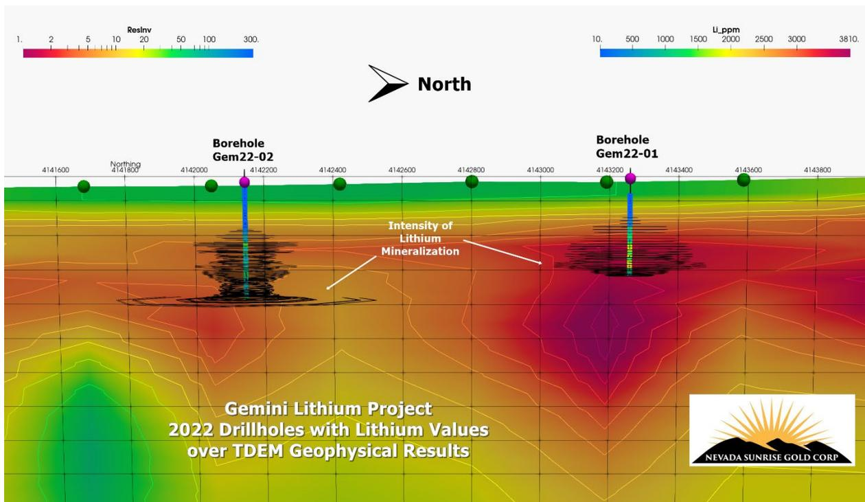
**Fig. 3: Gemini Lithium Project - Conductive Zone with 2022 Drillholes and Lithium Values**
