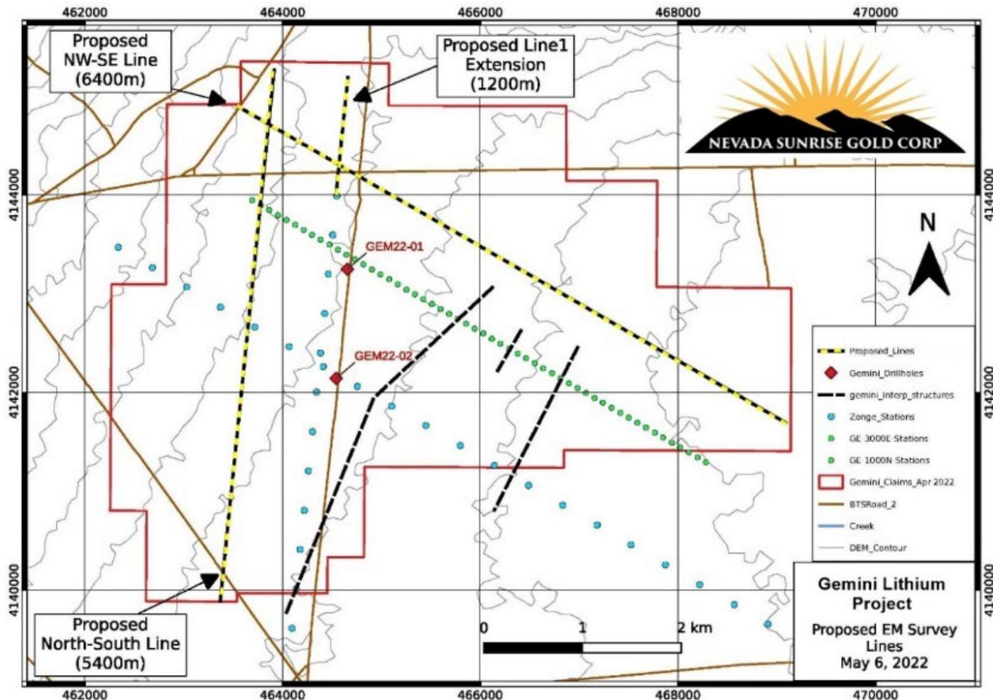
Fig. 2: Gemini Lithium Project 2022 TDEM Survey Plan
