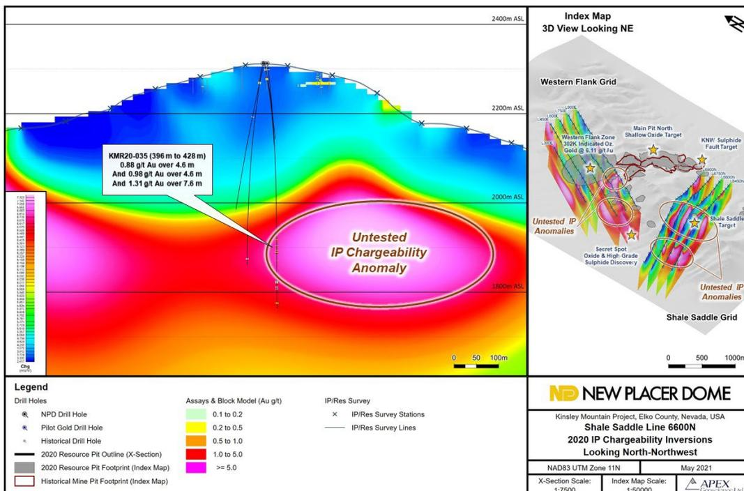
Figure 6. Shale Saddle Target IP Chargeability Section L6600N
