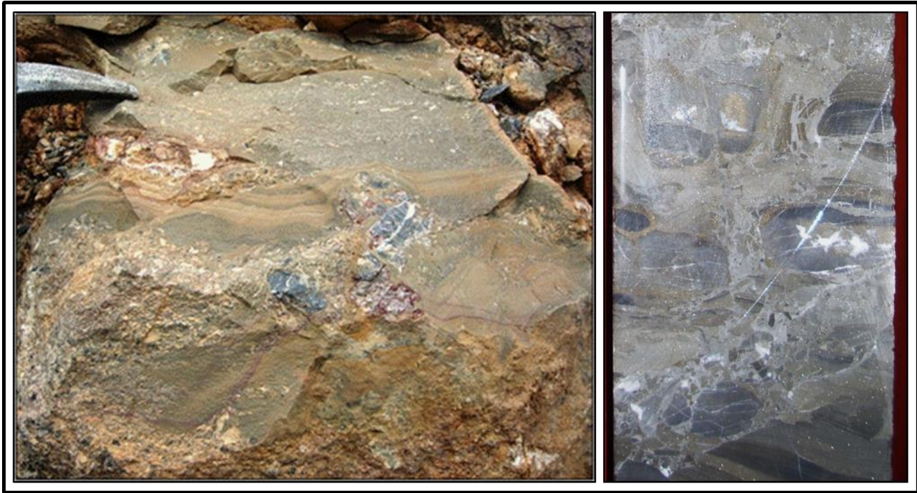
Left: Silicified cave fill breccia in Upper Pit. Note laminated geopetal fill draped over large limestone clasts in centre of photo. Right: Collapse breccia in high-grade interval, core hole PK91CA. Matrix/cement includes pyrite, silica and late calcite.
