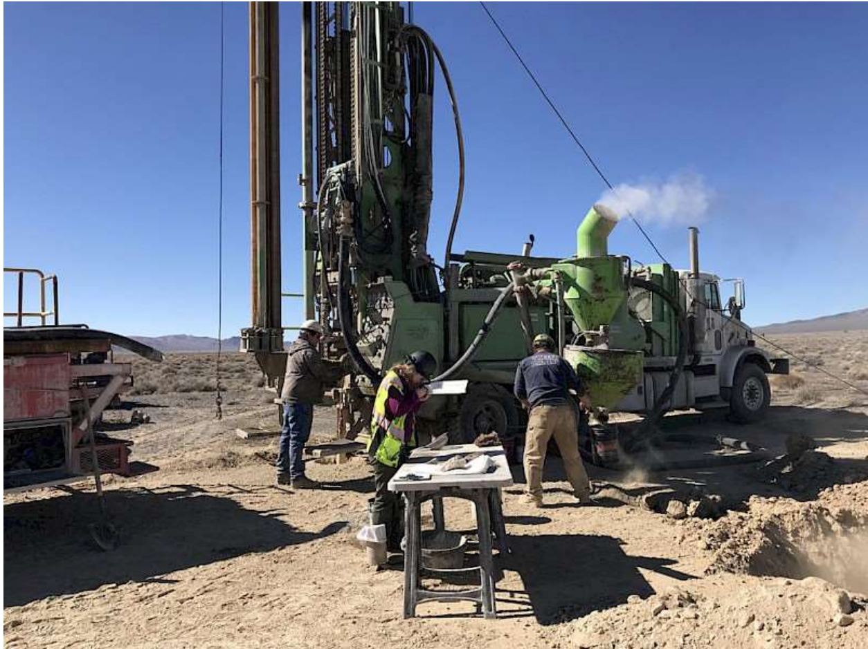
Figure 10-2: RC drilling, sampling with rotary splitter, geological logging of cuttings
